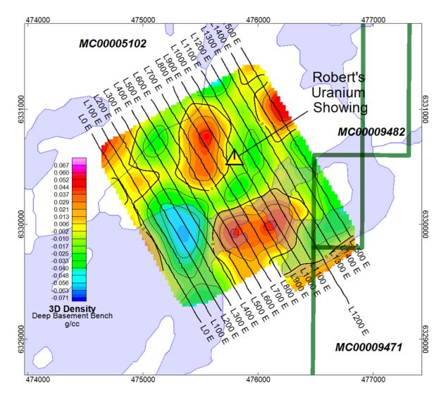
Figure 30: Gravity Inversion – Deep Basement Density Bench
