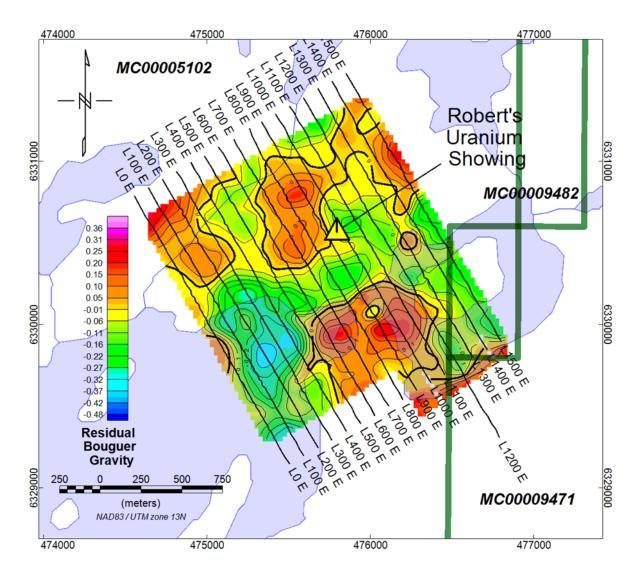
**Figure 25: Residual Bouguer Gravity**
