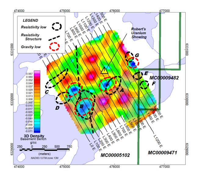
**Figure 32: Interpretation with Basement Gravity**
