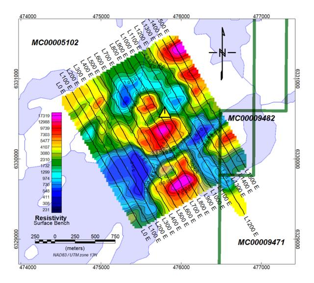
Figure 21: Resistivity - Near Surface Bench
