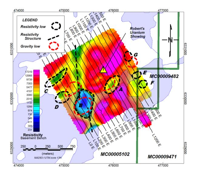
Figure 31: Interpretation with basement resistivity
