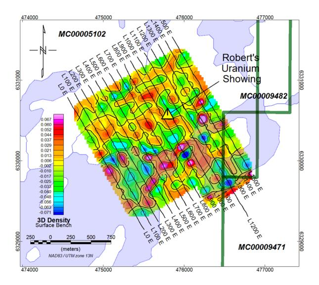
Figure 28: Gravity Inversion – Near Surface Density Bench
